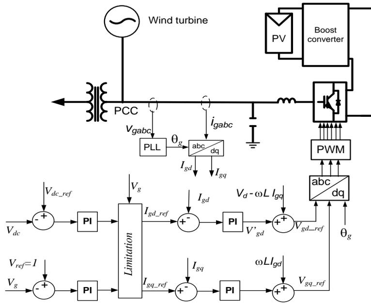
Fig. 4. Control diagram applying to the inverter.
