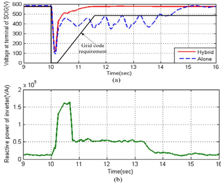
Fig. 8. Simulation results as two-phase fault: voltage at terminal of SCIG (a), PV system's reactive power (b)
