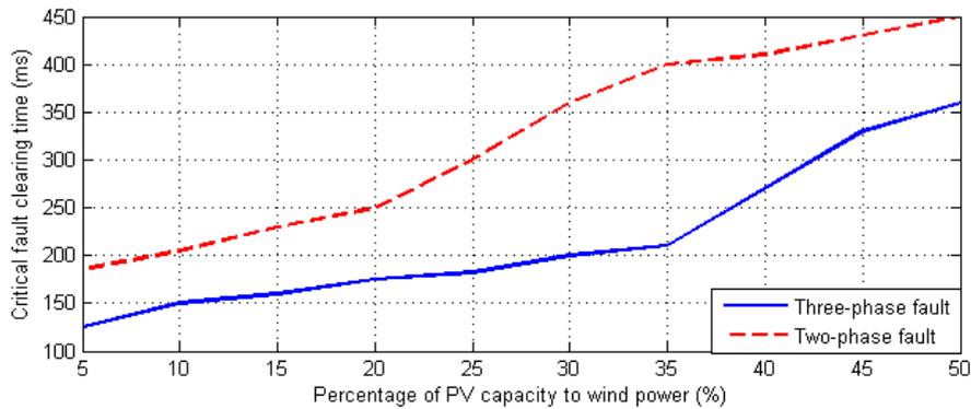
Fig. 9. Locus of critical fault isolating time with different PV capacity.
