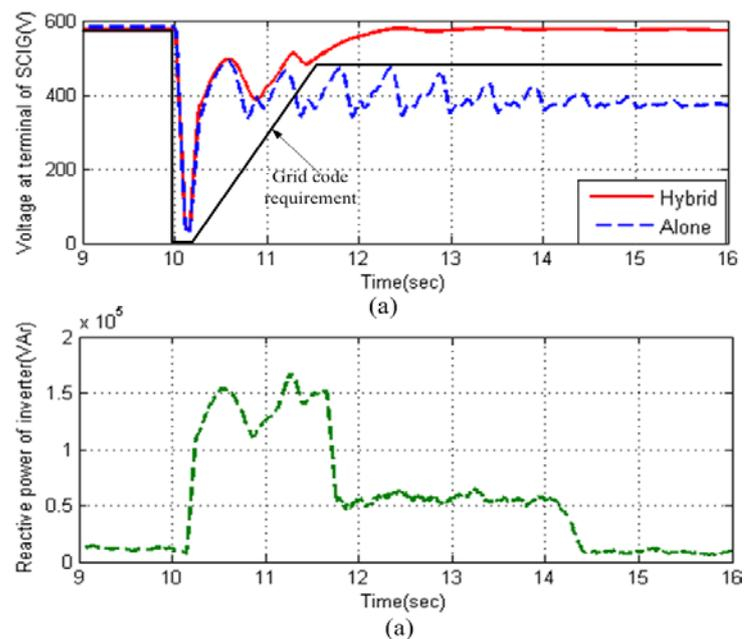
Fig. 7. Simulation results as three-phase fault: voltage at terminal of SCIG (a), inverter's reactive power (b).
