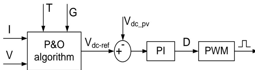
Fig. 3. Control diagram applying to the boost converter.
