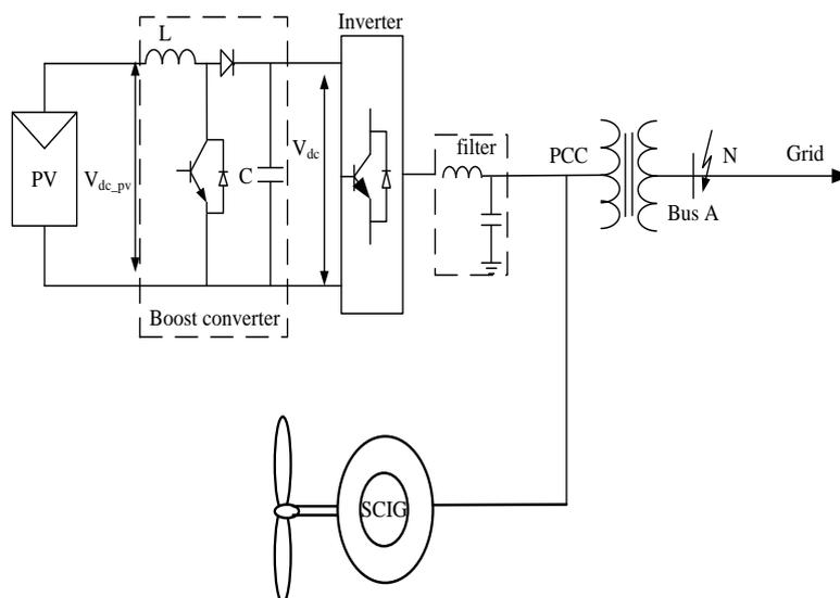
Fig. 1. Configuration a hybrid of PV and SCIG wind turbine.
