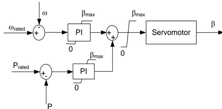
Fig. 2. Pitch control system of wind turbine.
