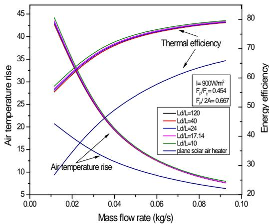
Fig. 13. Air temperature rise and energy efficiency as a function of mass flow rate for different flow length ratio.
