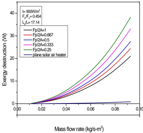
**Fig. 6. Exergy destruction as a function of mass flow rate for different fin spacing ratio.**
