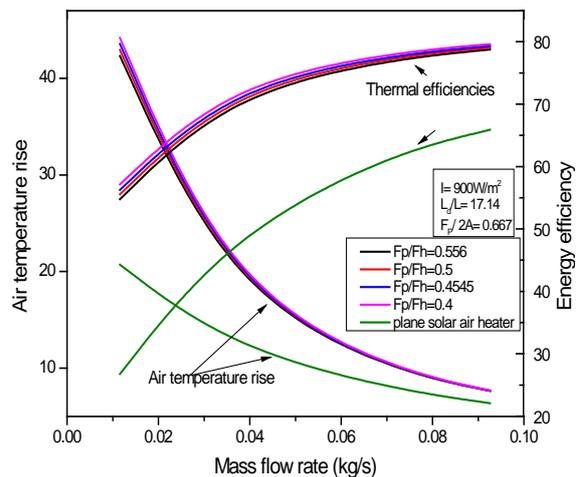
**Fig. 9. Air temperature rise and energy efficiency as a function of mass flow rate and different aspect ratio.**
