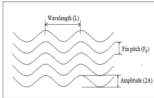
Fig. 2. Geometrical structure of wavy fin.
