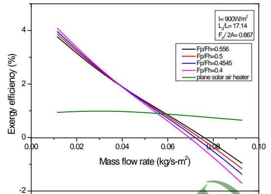
Fig. 11. Exergy efficiency as a function of mass flow rate for different flow cross section aspect ratio.
