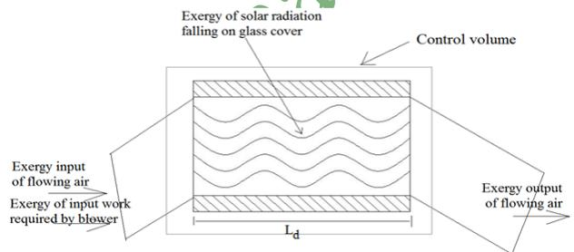
Fig. 3 (a). Exergy flow diagram of wavy finned solar air heater.
