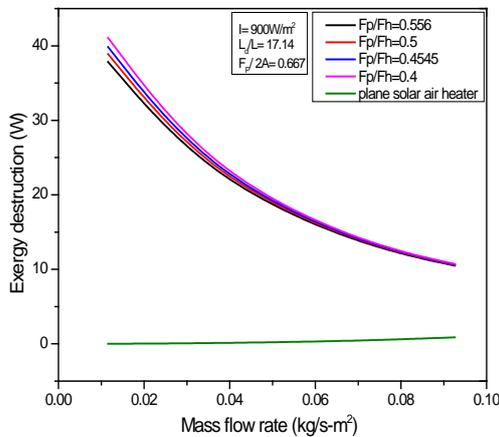
Fig. 10. Exergy destruction as a function of mass flow rate for different flow cross section aspect ratio.
