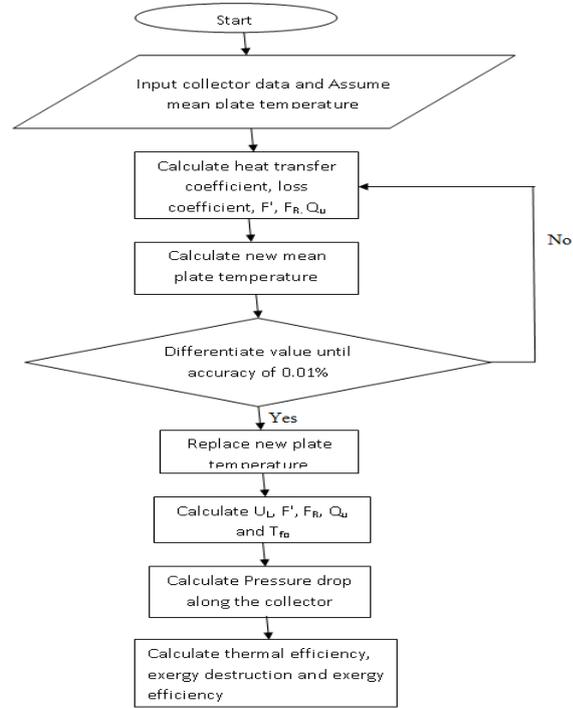
Fig. 3 (b). Flow chart for calculation of energy and exergy efficiency
