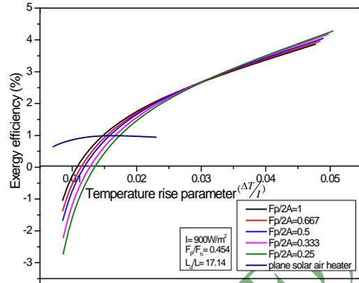
**Fig. 8. Exergy efficiency as a function of temperature rise parameter for different fin spacing ratio.**
