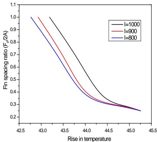
Fig. 17. Fin spacing ratio as a function of the air temperature rise for different insolation.
