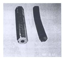
Fig.1 Commercially produced tropical wood sawdust briquettes before (left) and after (right) carbonization.
