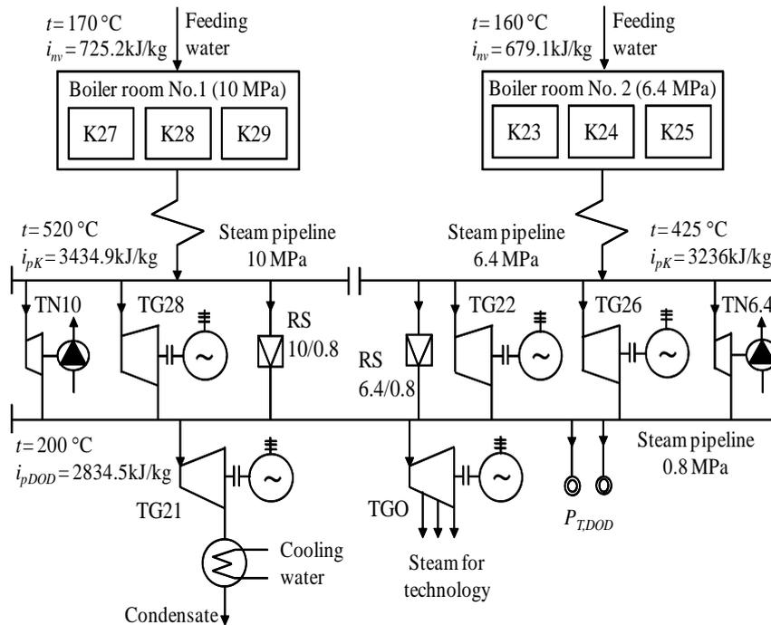
Fig. 2. Technological scheme of combined production of heat and electricity.
