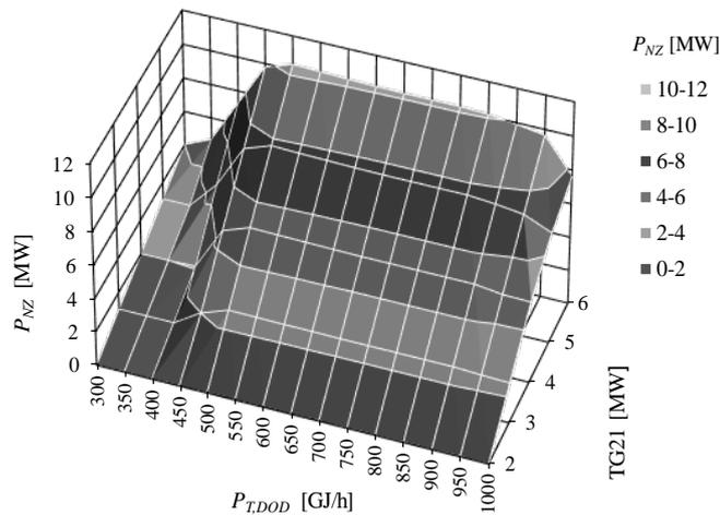
**Fig. 14. Output courses of independent electric output  $P_{NZ}=f(P_{T,DOD},TG21)$ ; heat supply  $P_{T,DOD} = 300 - 1000$  GJ/h with the step 50 GJ/h, electric output of TG21 = 2 - 6 MW with the step 1 MW.**
