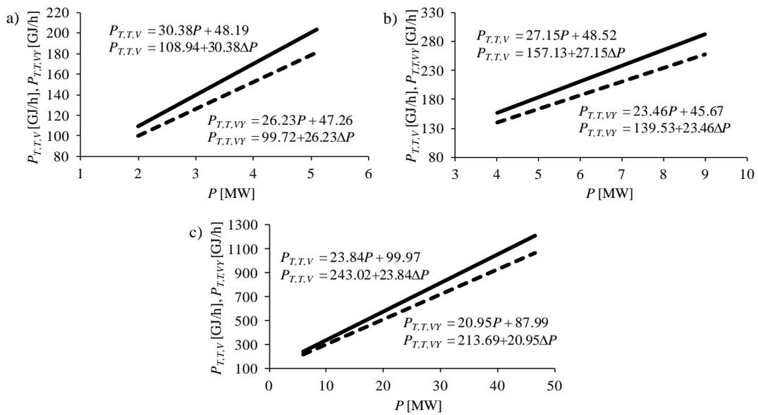
Fig. 7. Characteristics of back-pressure turbine: a) TG22, b) TG26 and c) TG28.
