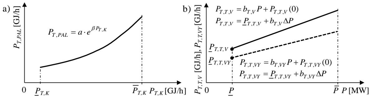
Fig. 3. Basic consumption characteristics: a) boiler, b) turbine.
