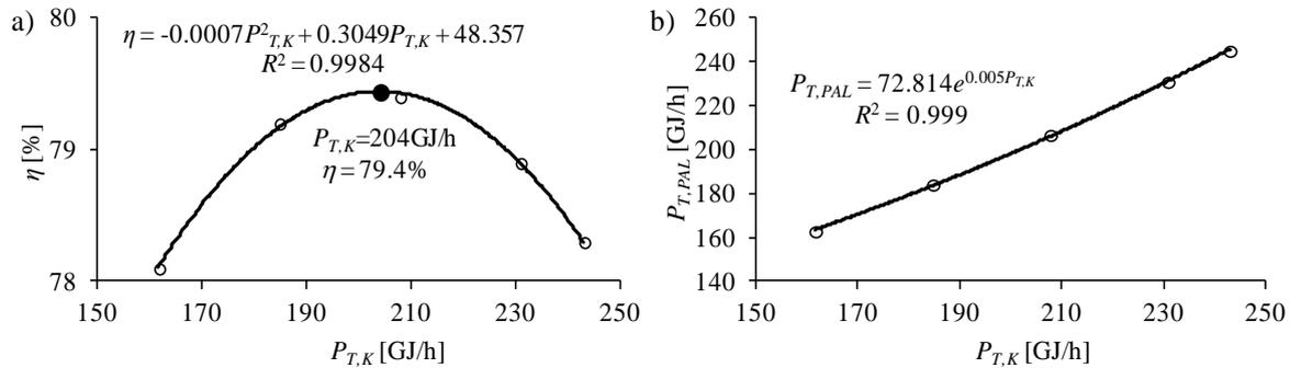
**Fig. 5. Characteristics of boiler K25: a) efficiency curve, b) consumption characteristic.**
