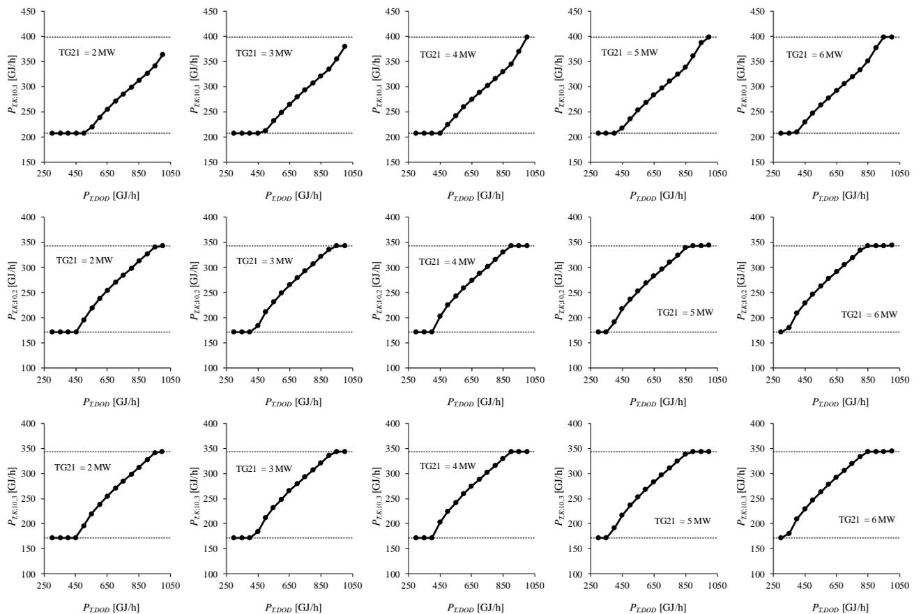
**Fig. 10. Optimal load distribution, between cooperating boilers K27, K28, K29, obtained via goal attainment algorithm for required values of electric output on TG21 and supplied heat output  $P_{T,DOD}$ .**
