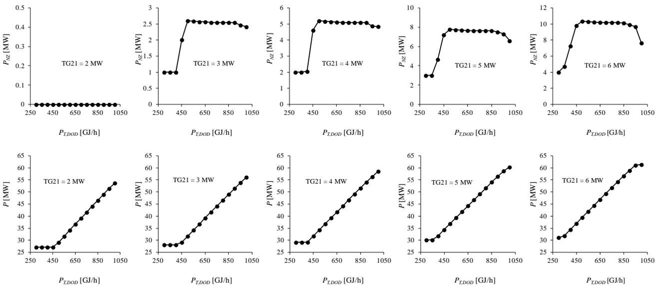
**Fig. 12.** Output courses independent electric output  $P_{NZ}$  and total produced electric output  $P$ , obtained by optimisation via goal attainment algorithm for required values of electric output on TG21 and supplied heat output  $P_{T,DOD}$ .
