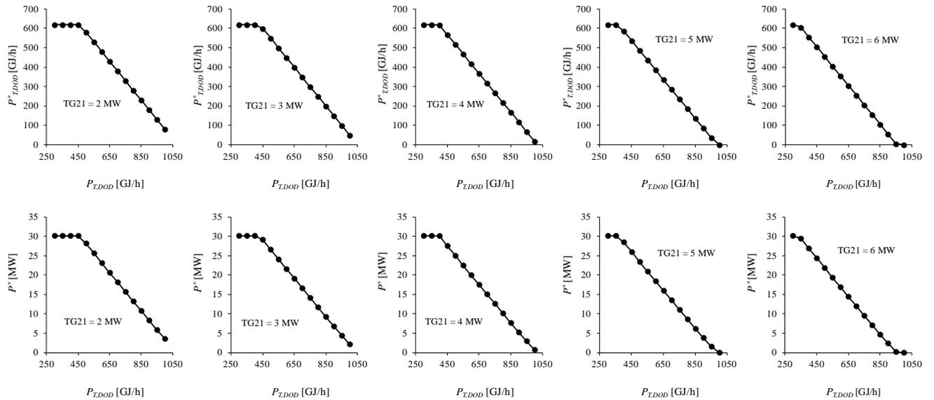
**Fig. 13. Output courses of reserve of heat output  $P^*_{T,DOD}$  and reserve of electric output  $P^*$  on individual back-pressure turbines TG22, TG26, TG28, obtained by optimisation via goal attainment algorithm at required values of electric output on TG21 and supplied heat output  $P_{T,DOD}$ .**
