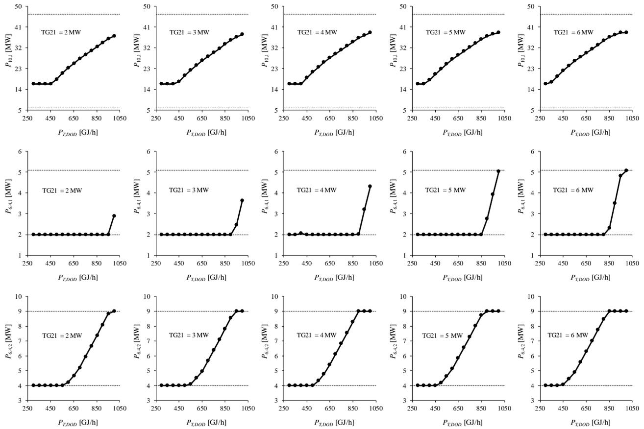
**Fig. 11.** Output courses electric output of individual back-pressure turbines TG28, TG22, TG26, obtained by optimisation via goal attainment algorithm for required values of electric output on TG21 and supplied heat output  $P_{T,DOD}$ .
