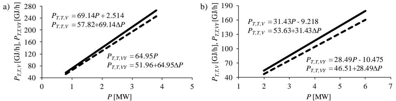
Fig. 8. Turbine characteristics: a) extraction steam turbine TGO, b) condensing turbine TG21.
