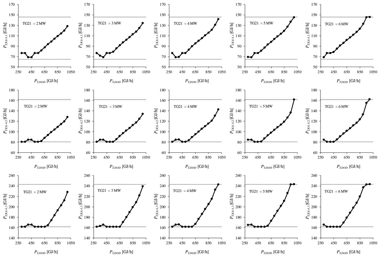
**Fig. 9. Optimal load distribution, between cooperating boilers K23, K24, K25, obtained via goal attainment algorithm for required values of electric output on TG21 and supplied heat output  $P_{T,DOD}$ .**
