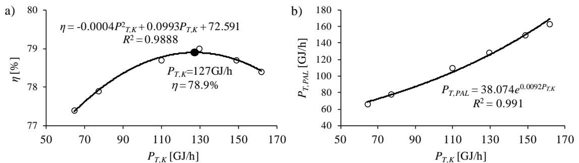
Fig. 4. Characteristics of boilers K23 and K24: a) efficiency curve, b) consumption characteristic.
