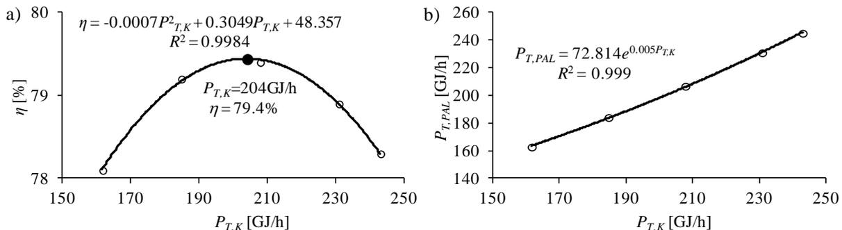
**Fig. 6. Characteristics of boilers K27, K28 and K29: a) efficiency curve, b) consumption characteristic.**
