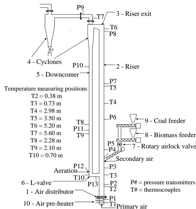
**Fig. 1. Schematic diagram of the CFB reactor.**
