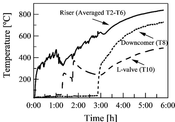
Fig. 2. Temperature in CFB reactor during start-up.
