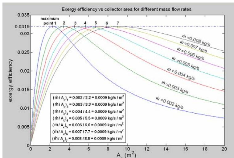
Fig. 6. Exergy efficiency versus collector area for different mass flow rates.
