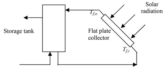
Fig. 3. A typical domestic scale solar water heater.
