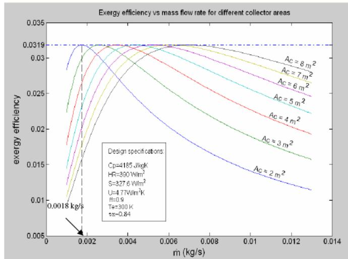
Fig. 5. Exergy efficiency versus mass flow rate for different collector areas.
