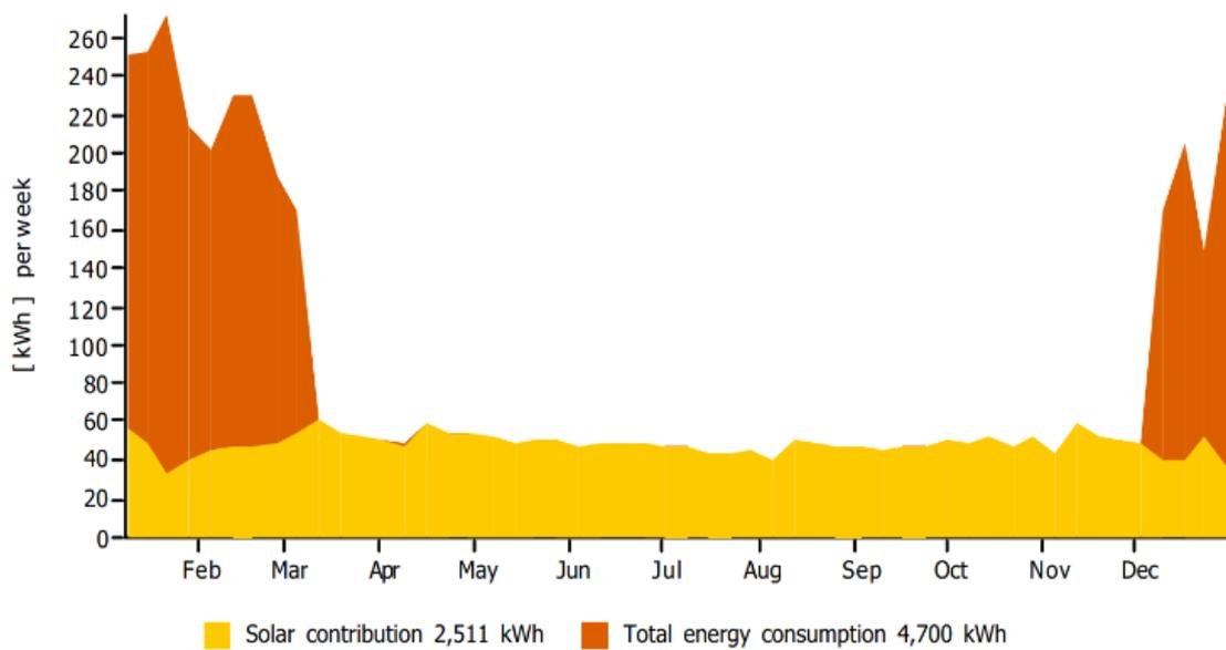
Fig. 2. Solar energy consumption in kWh of total consumption in Amman, Jordan from T\*SOL report for our four scenarios.
