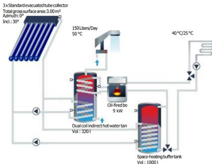
**Fig. 1. The simulated system's specifications and parts.**
