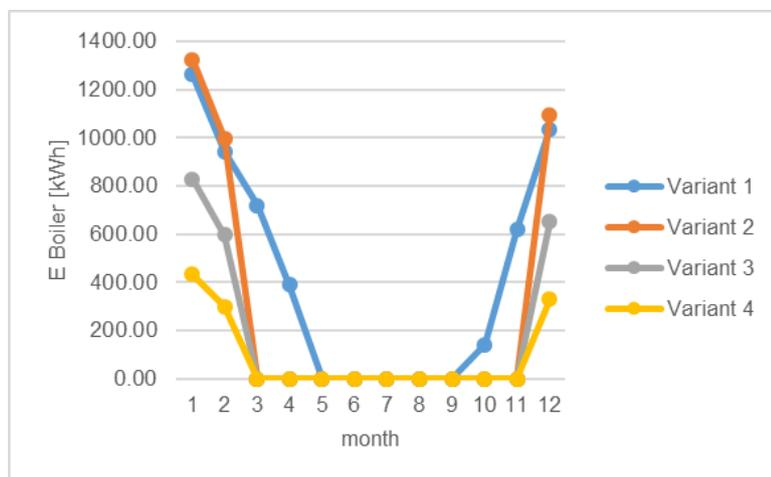
Fig. 8. Boiler energy utilization for heating in Amman, Jordan during 2022.
