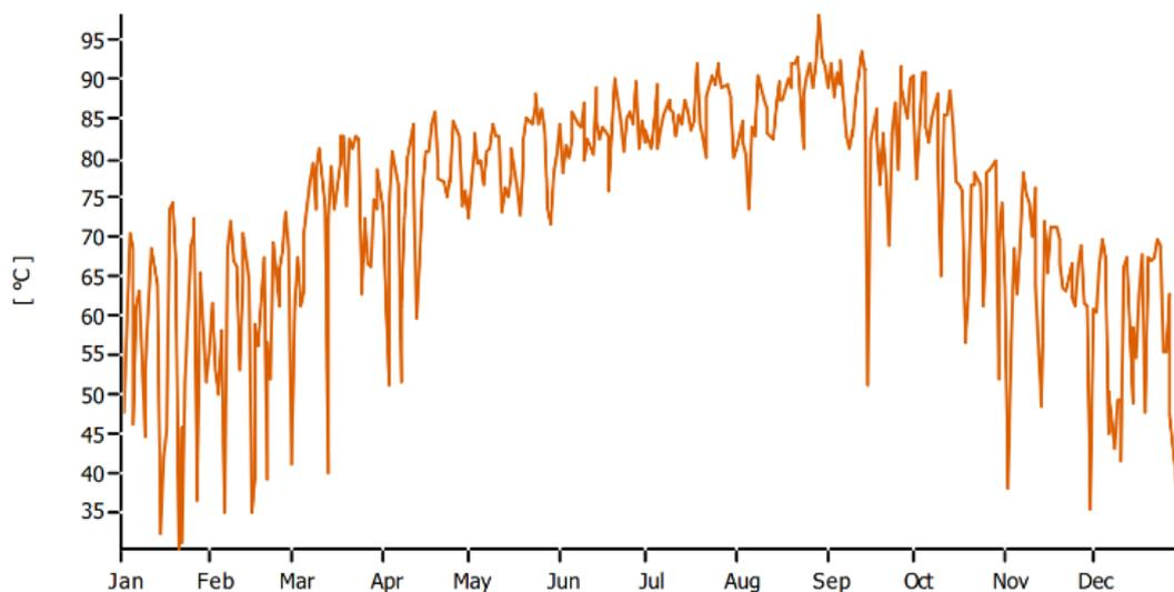
Fig. 3. Daily maximum collector temperature of a solar thermal collector in Amman, Jordan, showcasing the year-long trends in 2022.
