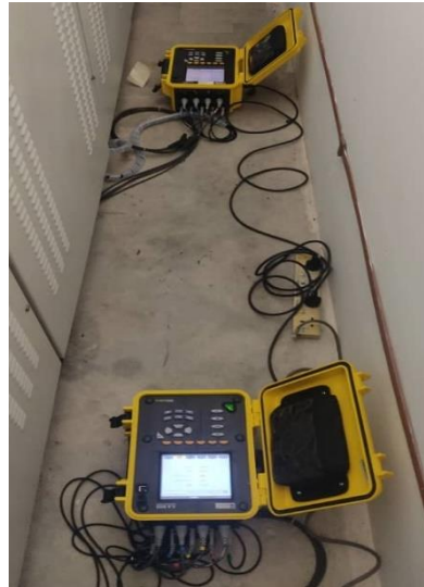
Fig. 4. Power logging process using power quality analyzers.
