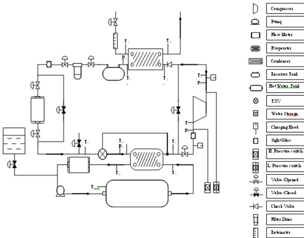
**Fig. 5. Schematic diagram of the experimental apparatus.**
