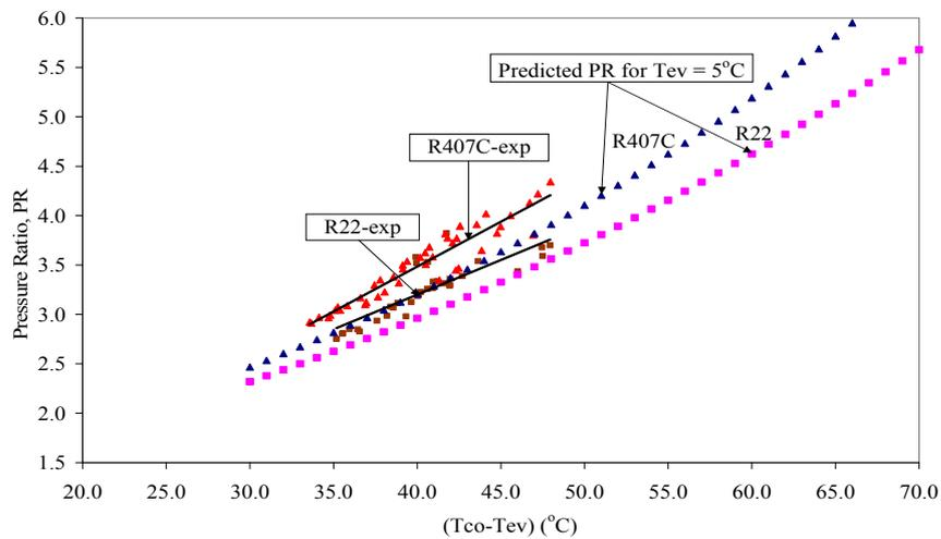
Fig. 10. Predicted and measured pressure ratio vs ( $T_{con}-T_{evap}$ ) for  $T_{ev}=5^{\circ}\text{C}$ .
