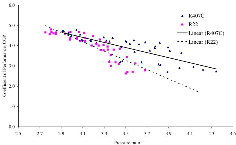
**Fig. 8. COP of heating vs. pressure ratio.**
