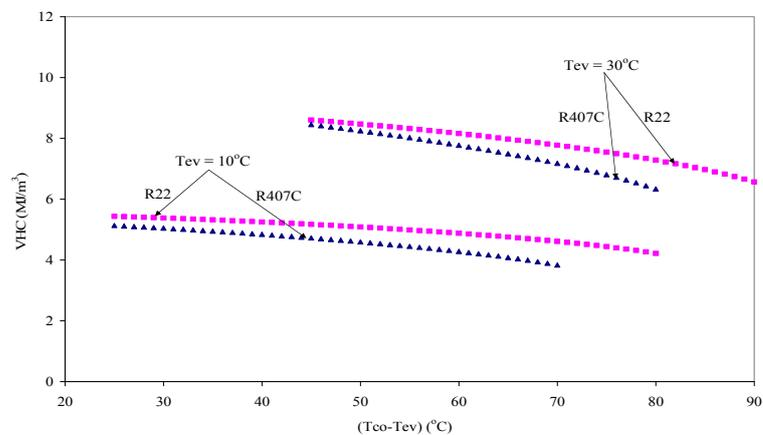
Fig. 3. VHC vs.  $(T_{CO}-T_{EV})$  for evaporating temperature,  $T_{EV}=10^\circ\text{C}$  and  $T_{EV}=30^\circ\text{C}$ .
