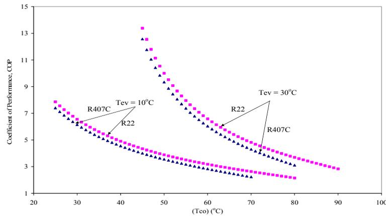
Fig. 2. Variation of COP vs.  $(T_{CO}-T_{EV})$  for evaporating temperature,  $T_{EV}=10^\circ\text{C}$  and  $T_{EV}=30^\circ\text{C}$ .
