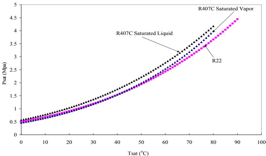
**Fig. 1. Saturation pressure vs. saturation temperature for different refrigerants.**
