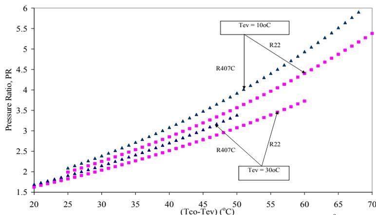
Fig. 4. Pressure ratio vs.  $(T_{CON}-T_{EVAP})$  for evaporating temperature  $T_{EV}=10^\circ\text{C}$  and  $T_{EV}=30^\circ\text{C}$ .
