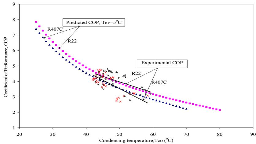
Fig. 9. Predicted and measured COP vs. ( $T_{co}$ ) for evaporating temperature  $T_{ev}=5^{\circ}\text{C}$
