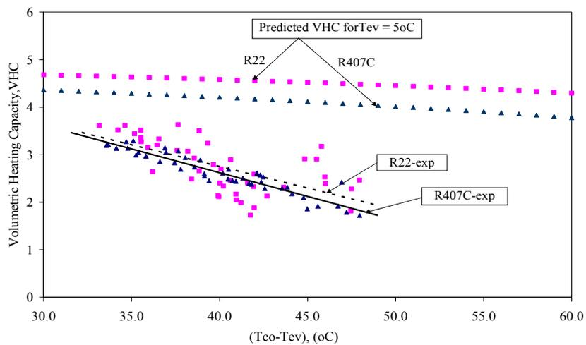
Fig. 11. Predicted and measured VHC vs. ( $T_{co}-T_{ev}$ ) for  $T_{ev}=5^{\circ}\text{C}$ .
