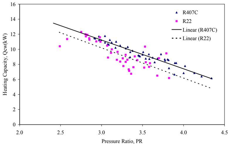
**Fig. 6. Heating capacity vs. pressure ratio.**
